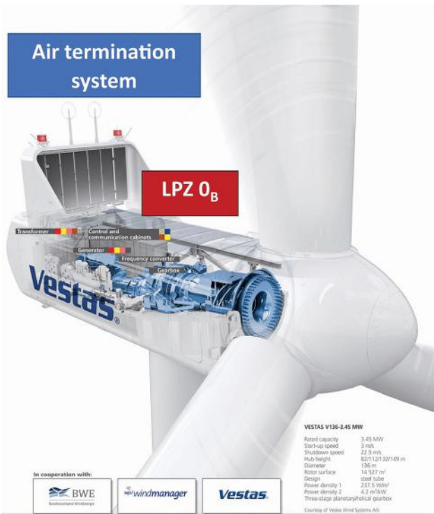
Figure 3: Air termination systems installed for wind turbine nacelle
