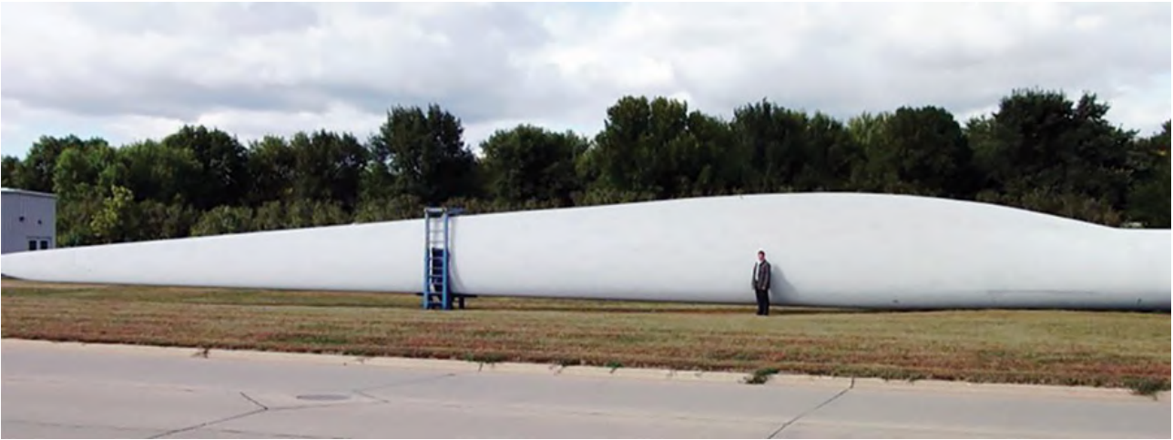
Figure 9: Wind turbine blade before installation
