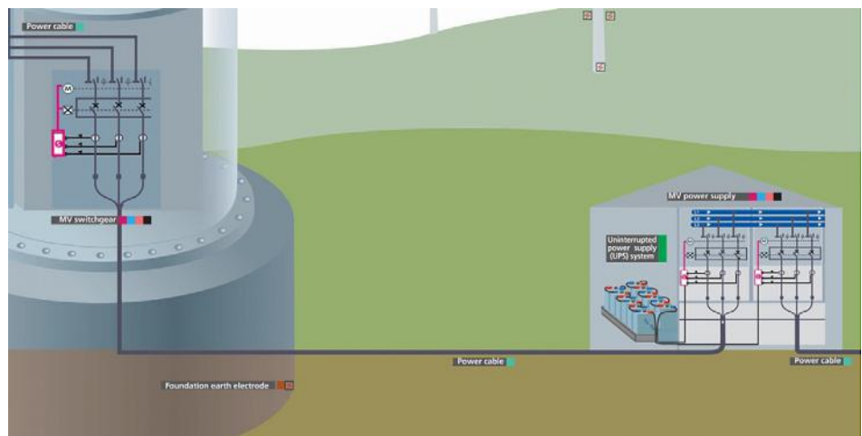
Figure 5: Foundation earth electrode at wind turbine base
